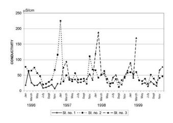
Fig. 3. Monthly pattern of conductivity in open area.
